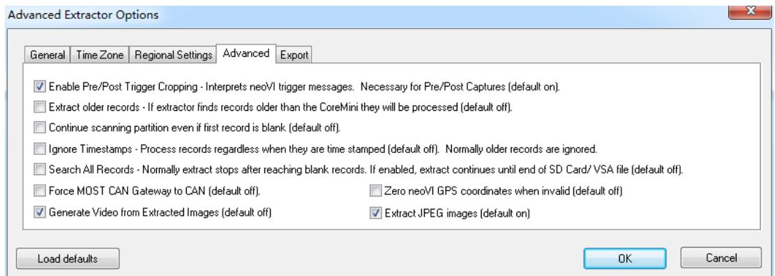
Figure 9: Advanced settings to generate video from the logged data.
