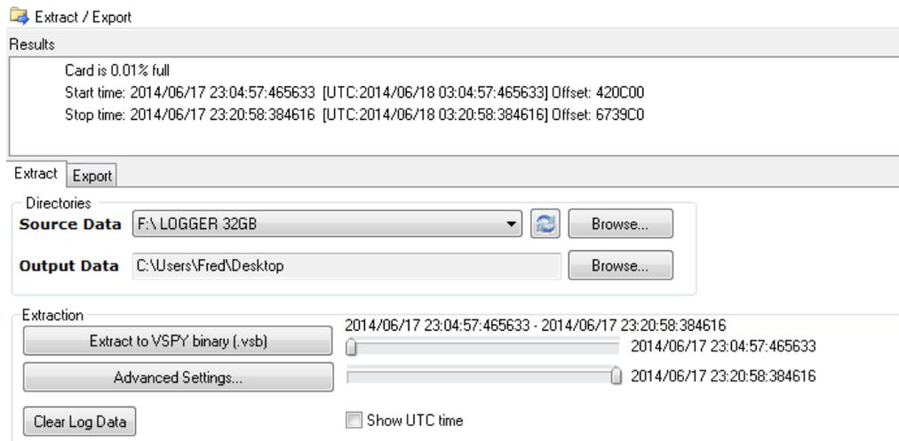
Figure 8: Extractor settings to extract the logged files from the SD Card
