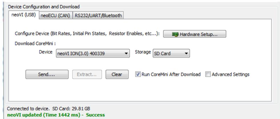
Figure 7: VehicleScape DAQ settings to download CoreMini executable in ION
