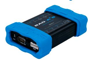
RAD-A2B combines Analog Devices' A2B technology with two CAN/CAN-FD transceivers and one LIN channel to allow mixed network messages in one time stamped log. The RAD-A2B tool includes one channel for A2B receive-only monitoring and one channel that can act as an emulator node.
