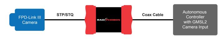
Power-over-coax as pass-thru or supply to camera / sensor.
