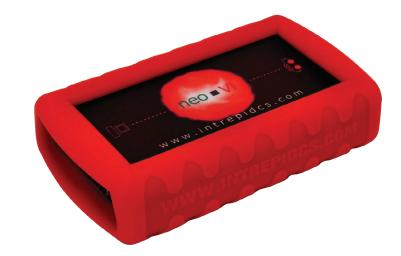
channels become standard, you can rely on the neoVI RED, with its accuracy of 10 microseconds, to monitor CAN and LIN networks without missing a message.
