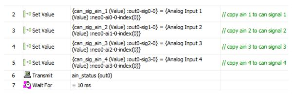
Optionally, if you used a variable and read the analog input port into a variable then you would assign the variable to the appropriate CAN signal as shown below.
