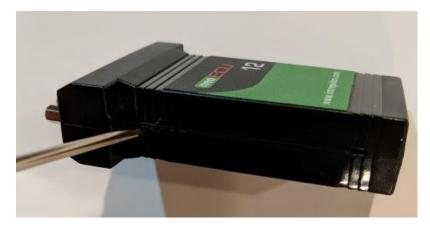
Press and hold one of these switches to get in that particular mode when applying power to the neoECU-12. After power is applied the LEDs will light red in sequence from 1 to 5 and repeat.
