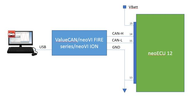
Termination. Please note the neoECU-12 does not have built-in selectable termination resistors. Therefore, an external resistor (120 ohm) is required on the CAN-H and CAN-L pins as shown below. The device you are connecting to also needs the termination resistor. Most of the Intrepid Control System devices have built-in selectable termination resistors that can be enabled in via the hardware setup for that device. If this option is not available, then add the external resistor as shown below.
