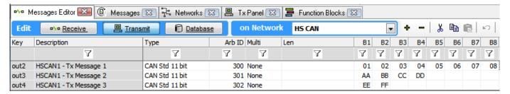
In the Tx Panel set the rate to be 100 ms and periodic. This is a test only. The ECU will have it's own rates for each message or you can duplicate the rates here.
