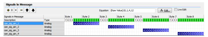
Next modify the script to get the analog in value and copy it into its respective CAN signal. In this example the port is read and directly copied into the CAN signals then the CAN message is sent every 10 ms.
