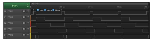
Note: The PWM output is 3.3V signal driven by a series 10K resistor. Please buffer accordingly to drive higher current loads.
