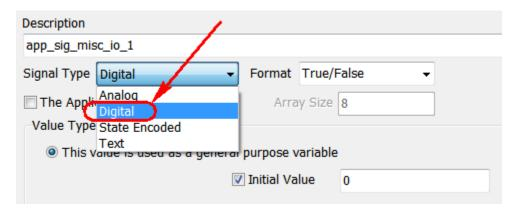
Do this for the remaining MISC IO inputs. Note the Format is defaulted to "True/False" but you can switch to "On/Off", "Yes/No", "Passed/Failed", "Open/Closed", etc...
