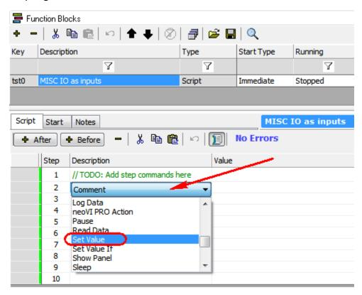
Next click on the empty cell row 2 column Value. Note the red text "The SetValue expression could not compile" message. Please note all error messages needs to be corrected before the script can be compiled and programmed into CoreMini. Once we set the value correctly the error message will go away.
