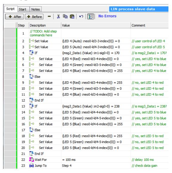
Also note for this example the "LIN Master msg2" and "LIN Master msg3" were copied from the Transmit table and added to the Receive table. Then "msg2\_Data1" thru "msg2\_Data4" signals and "msg3\_Data1" thru "msg3\_Data2" signals were added to their respective messages. The signals needed to be defined so they could be processed in the script.
