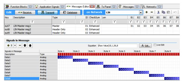
If we program this example into the neoECU-12 and then use another Intrepid device to monitor the LIN Bus these are the messages on the LIN Bus. Note there is an error for LIN message "LIN 02" and "LIN 03". This is because the monitoring or slave device has not sent back any data to the LIN Master (neoECU-12).
