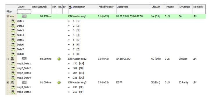
To see the LIN columns in the message view select LIN from the Columns button at the bottom of the messages view.
