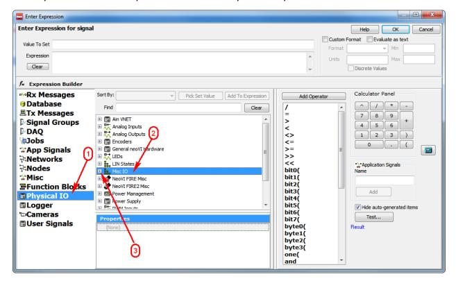
Next click on "MISC IO 1" followed by double-clicking on the "IS Output" property. This adds MISC IO 1 (Is Output) to the "Value to Set" box. Then put "0" for the Expression and click the OK button. "0" = input and "1" = output.
