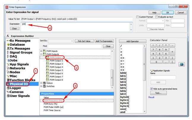
Continue setting the PWM Output 2 thru 5 to 100Hz as shown below.
