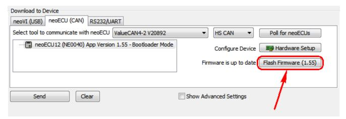
After the device is successfully updated you will see that it no longer shows "Bootloader Mode" and LED 3 is blinking a magenta color. During the flash sequence LED 3 blinks an orange color.
