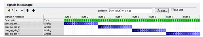
Or re-size the 16-bit signal values to 12-bit values by dragging the edge of the blue box inwards.
