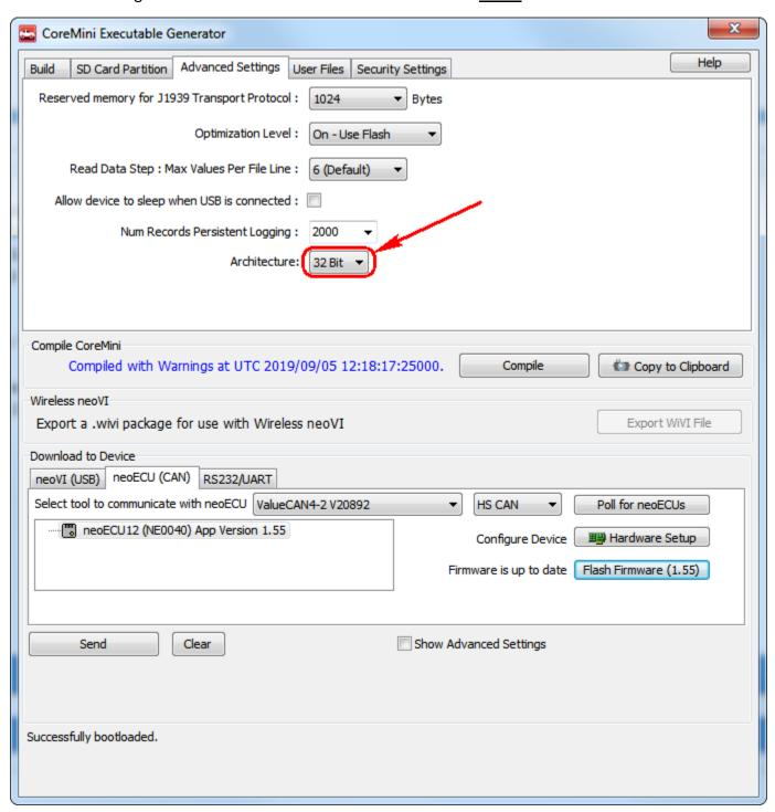
After selecting 32-bit click back to the Build tab. Click on the "Compile" button, followed by clicking on the "Clear" button, followed by clicking on the "Send" button. Once the progress bar is complete you have programmed the CoreMini of the device. The message at the bottom of the screen will show "Successfully downloaded" and the neoECU 12 shows "Running CoreMini".
