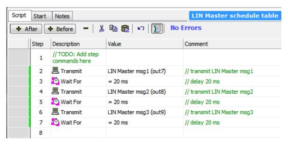
In this example, three LIN Transmit messages were created. "LIN Master msg1" is a message that contains data that will be sent to the LIN slaves. The signals were pre-defined as "01" thru "08" but can be modified in the script. The signals in "LIN Master msg1" were named "Data1" thru "Data8" as shown below. Note the Type is "Master". For LIN messages that will contain data from the slaves the Type needs to be set to "Header Only".
