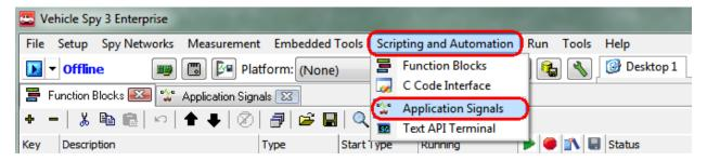
Next click on the "+" symbol to add "Application Signals". These are like variables in C code. Clicking on the "+" symbol again to add additional application signals and clicking on the "-" symbol will delete the application signal that is highlighted.
