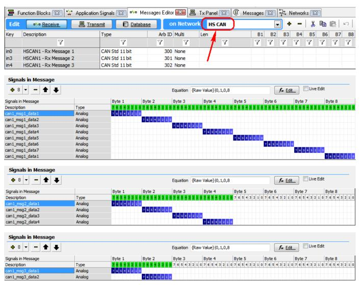
Create 3 HS CAN 2 Transmit messages and their respective signals as shown below. Hint: go to the HS CAN 1 Receive table and copy the 3 messages. Then go to the HS CAN 2 Transmit table and paste the messages. Paste into the Description column. This will copy over the signals as well! Change the Type to "CAN FD Std 11 bit" for all 3 messages.
