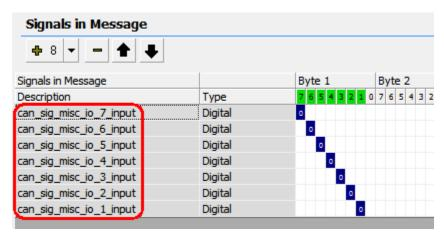
Next modify the script to get the MISC IO port value and copy it into its respective CAN signal. In this example the port is read and copied into the CAN signals then the CAN message is sent every 50 ms.
