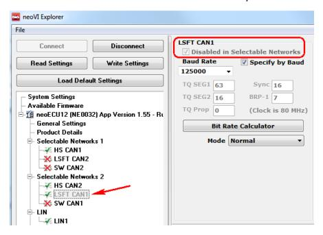
The best method for selecting the network is to click on "Selectable Networks 1" or "Selectable Networks 2" and from the pull-down menu make your selection.
