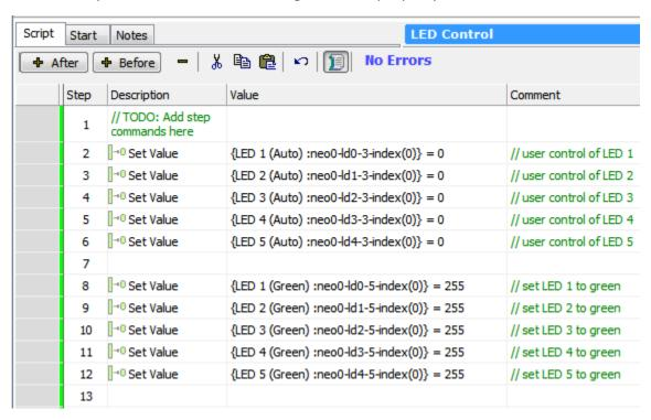
The proper way to set the LED color is to assign values to the red/green/blue property. This example shows how to set LED 1 to green color.
