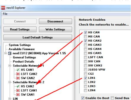
In this example you can see HS CAN 1, HS CAN 2, and LIN is enabled.
