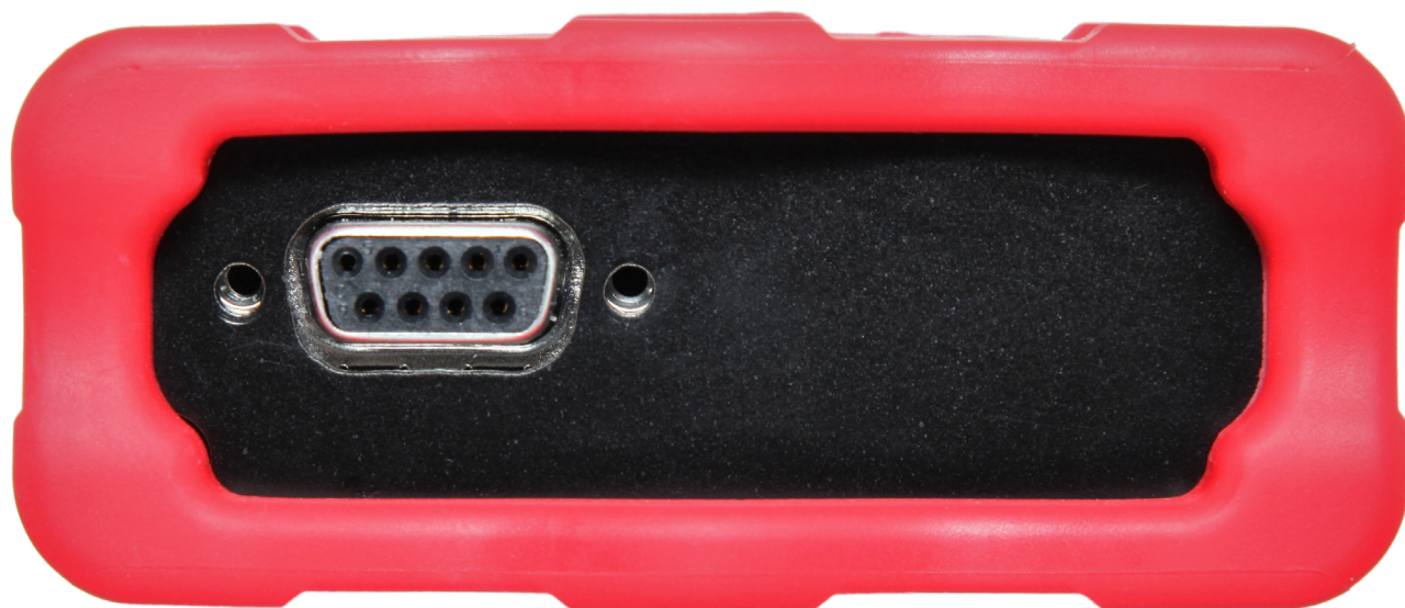
Figure 4: Right Side of neoVI Flex. This side of the device contains just a single female DB-9 connector, reserved for future use.
