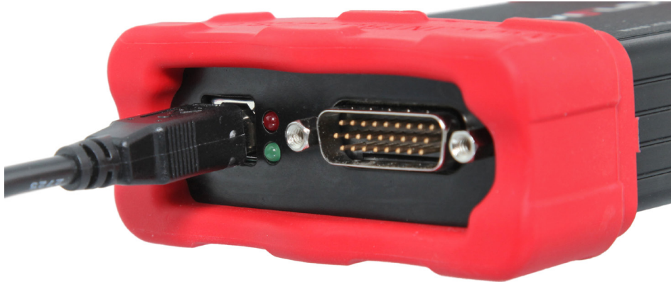
Figure 9: Connecting the USB cable to the neoVI FLEX.
