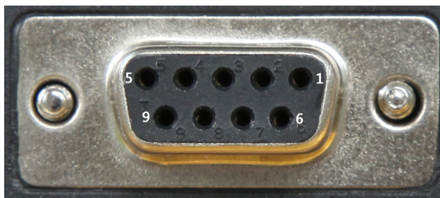
Figure 7: Data Cable DB-9 Connector. Note that the pin numbers are actually imprinted right on the connectors, but they can be hard to see, so we have labeled the edge pin numbers here.
