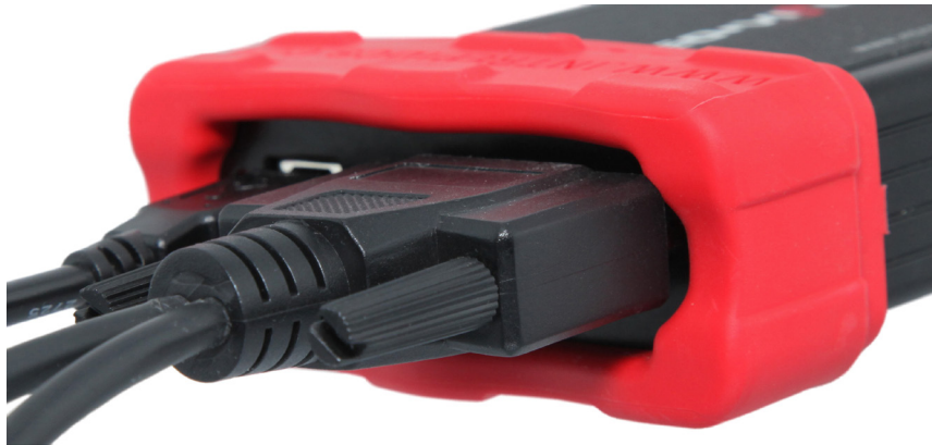
Figure 10: Connecting the data cable to the neoVI FLEX.
