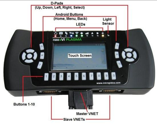
Figure 2: Features on the front and bottom of neoVI PLASMA.
