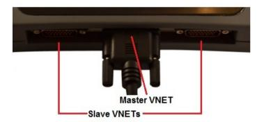
Figure 1: neoVI PLASMA has 3 VNET connections along the bottom.
