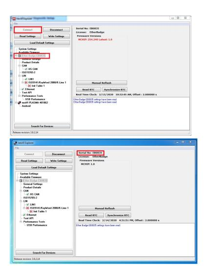
Once the hardware is connected please press the **Manual Reflash** button to update the firmware, you might have to press the update button twice.
